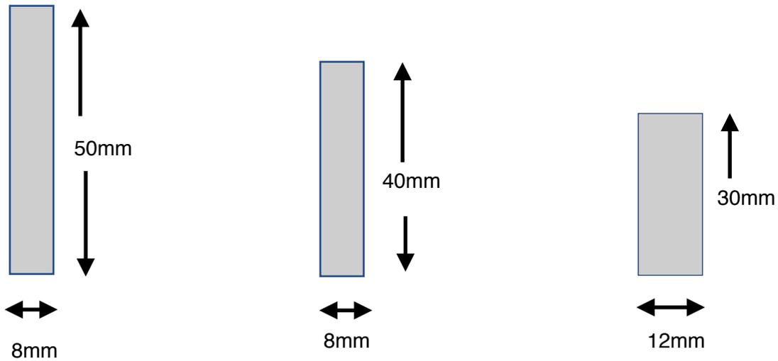
Rail variations given above. The Rail is reusable. Above photograph gives example of a rail been moved during concrete pour to new position into pre set Rail Supports.
