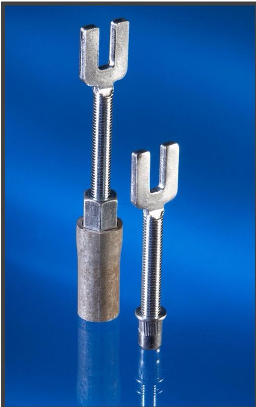
There are two plugs as shown in the image to the left. The small plug is used for depths up to 75mm and the large plug for slabs of greater depths above 75mm. A hole is drilled into the existing concrete and we suggest spacings are 1 meter apart. The small plug requires a 12mm hole and the large plug a 20mm diameter hole. The depth of the whole drilled determines the adjustment range during set up.
